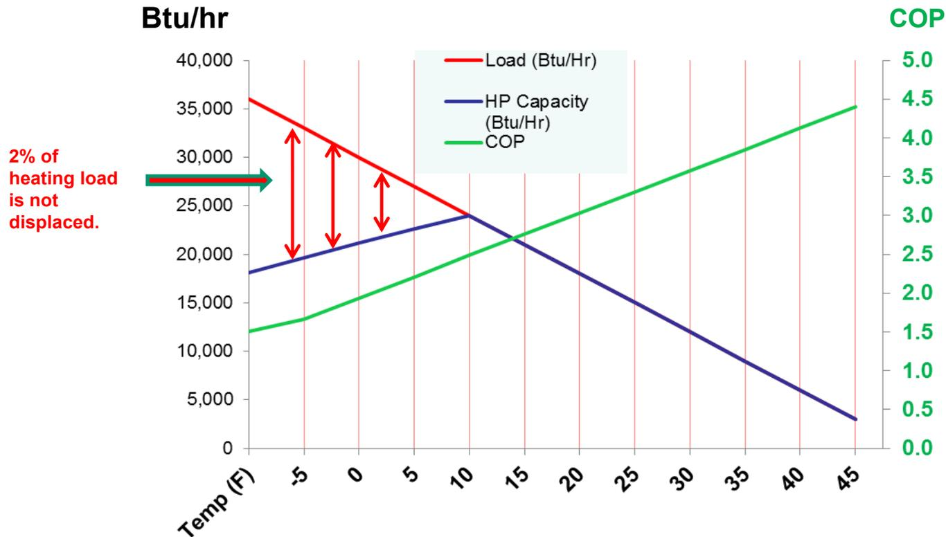
COP decreases with outdoor temperature. Supplemental heating typically required for DSHP at low outdoor temperatures. However, most (sometimes all) of load is covered with DSHP.
