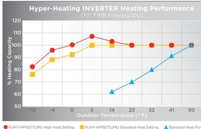
Greatly improved performance. However, supplemental heating may be required for low outdoor temperatures. However, most (sometimes all) of load can still be met. Shell upgrades can help eliminate the gap.
